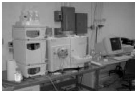
New Finnigan LCQ DECA tandem (MS-MS) mass spectrometer with an ion trap and capability to select and analyze fragments from the parent ion.
